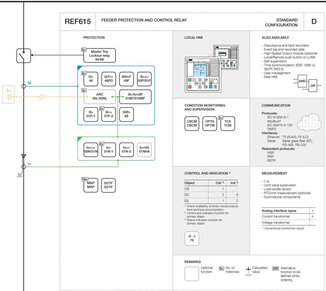
Figure 4. Functionality overview for standard configuration D
