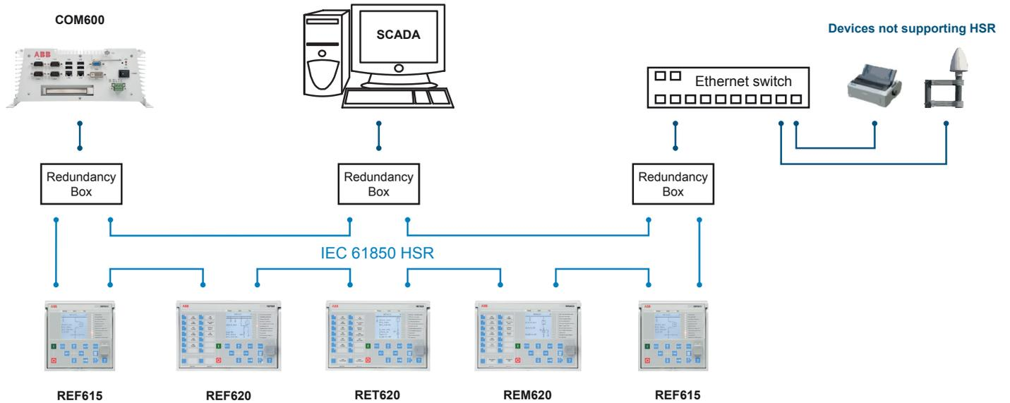
Figure 23. High availability seamless redundancy (HSR) solution
