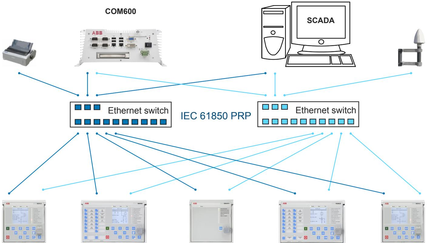
Figure 22. Parallel redundancy protocol (PRP) solution
