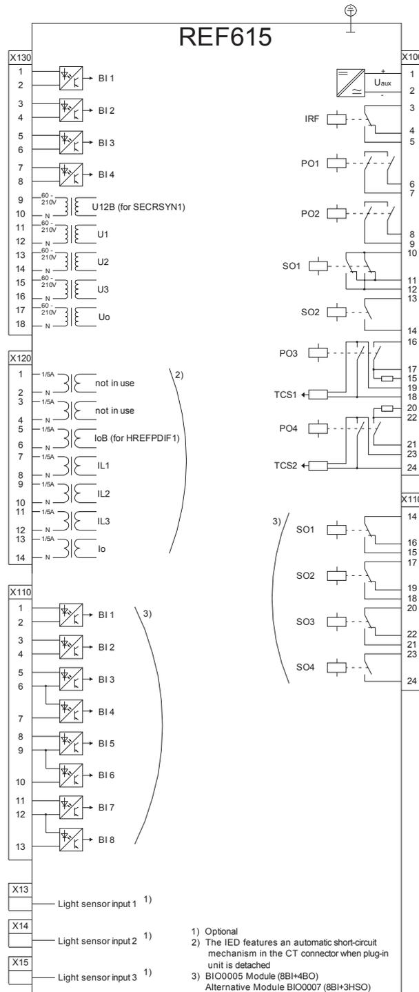
Figure 35. Terminal diagram of standard configuration K
