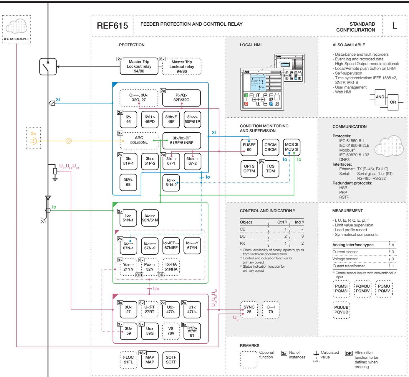
Figure 11. Functionality overview for standard configuration L
