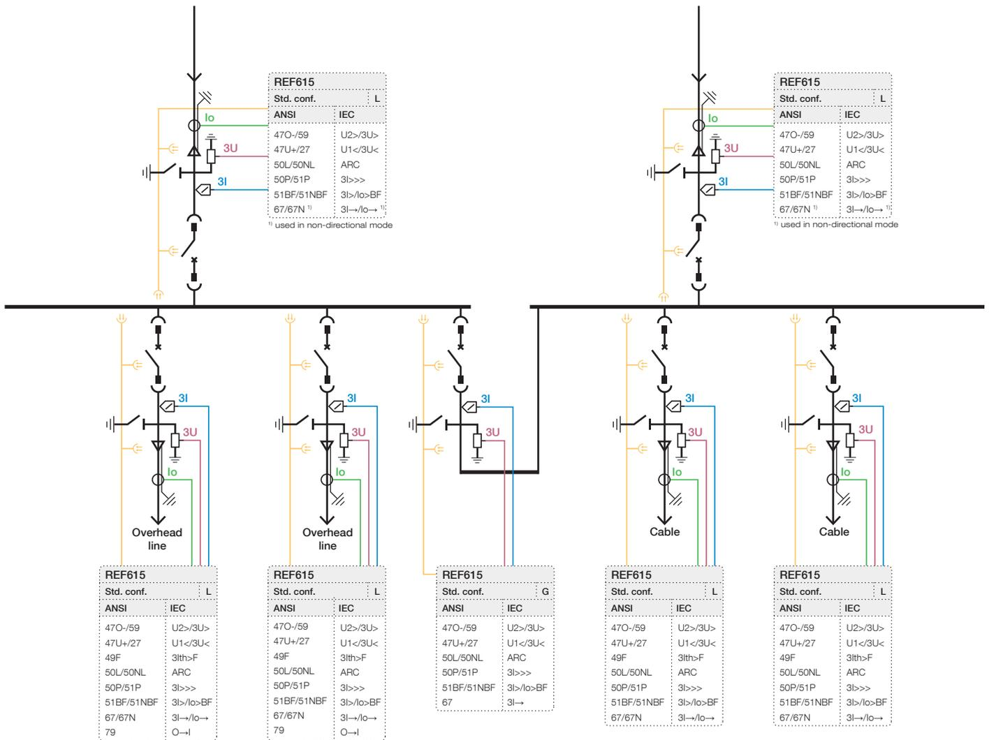
Figure 15. Application example with single busbar switchgear arrangement
