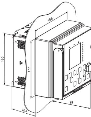
Figure 28. Semi-flush mounting
