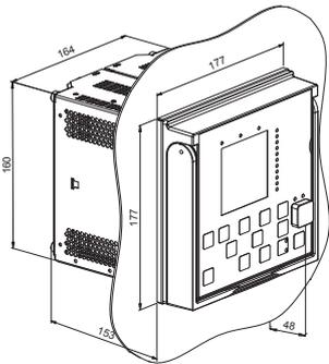
Figure 27. Flush mounting
