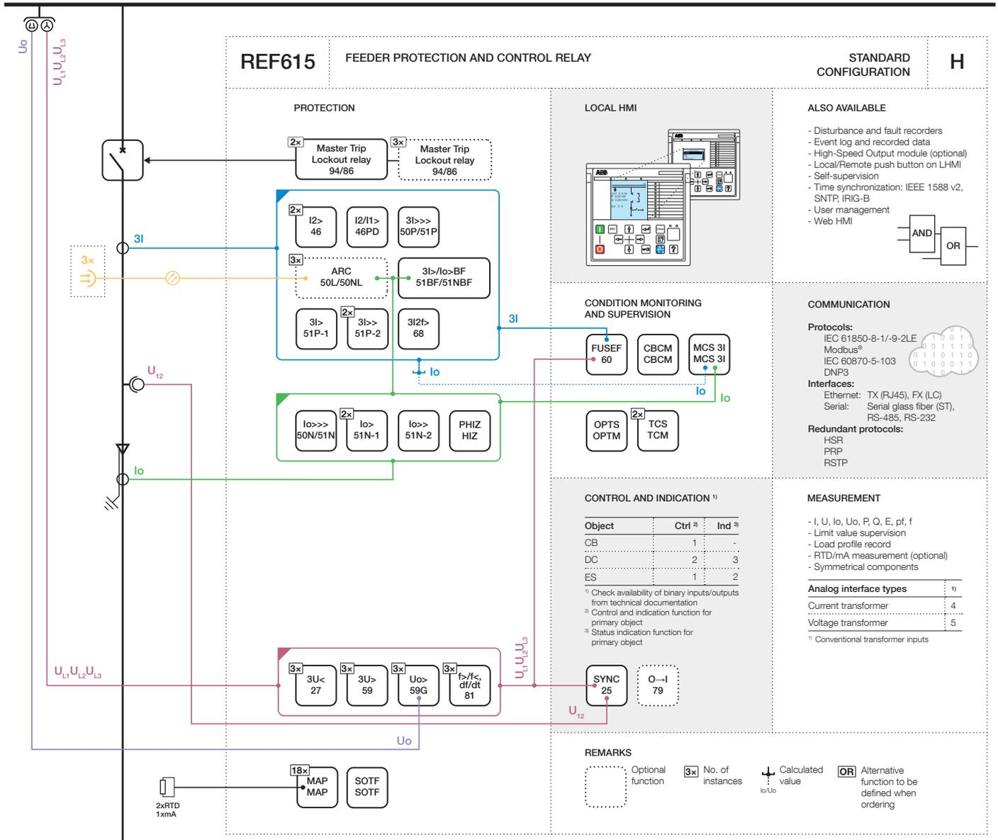
Figure 8. Functionality overview for standard configuration H
