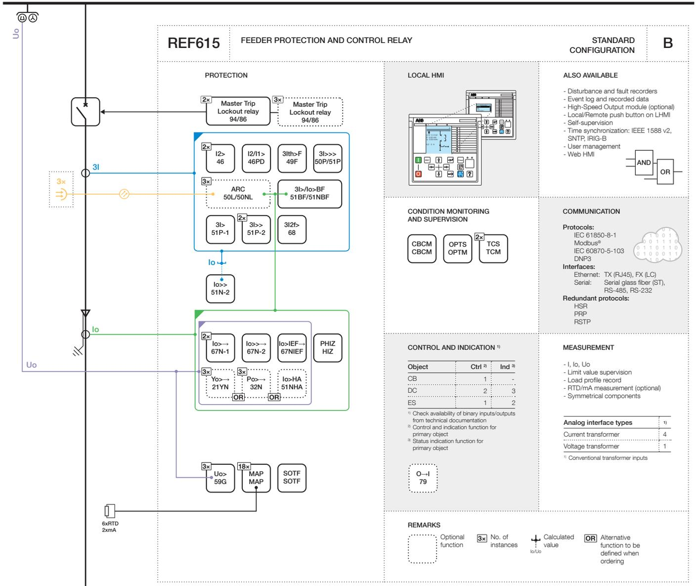
Figure 2. Functionality overview for standard configuration B
