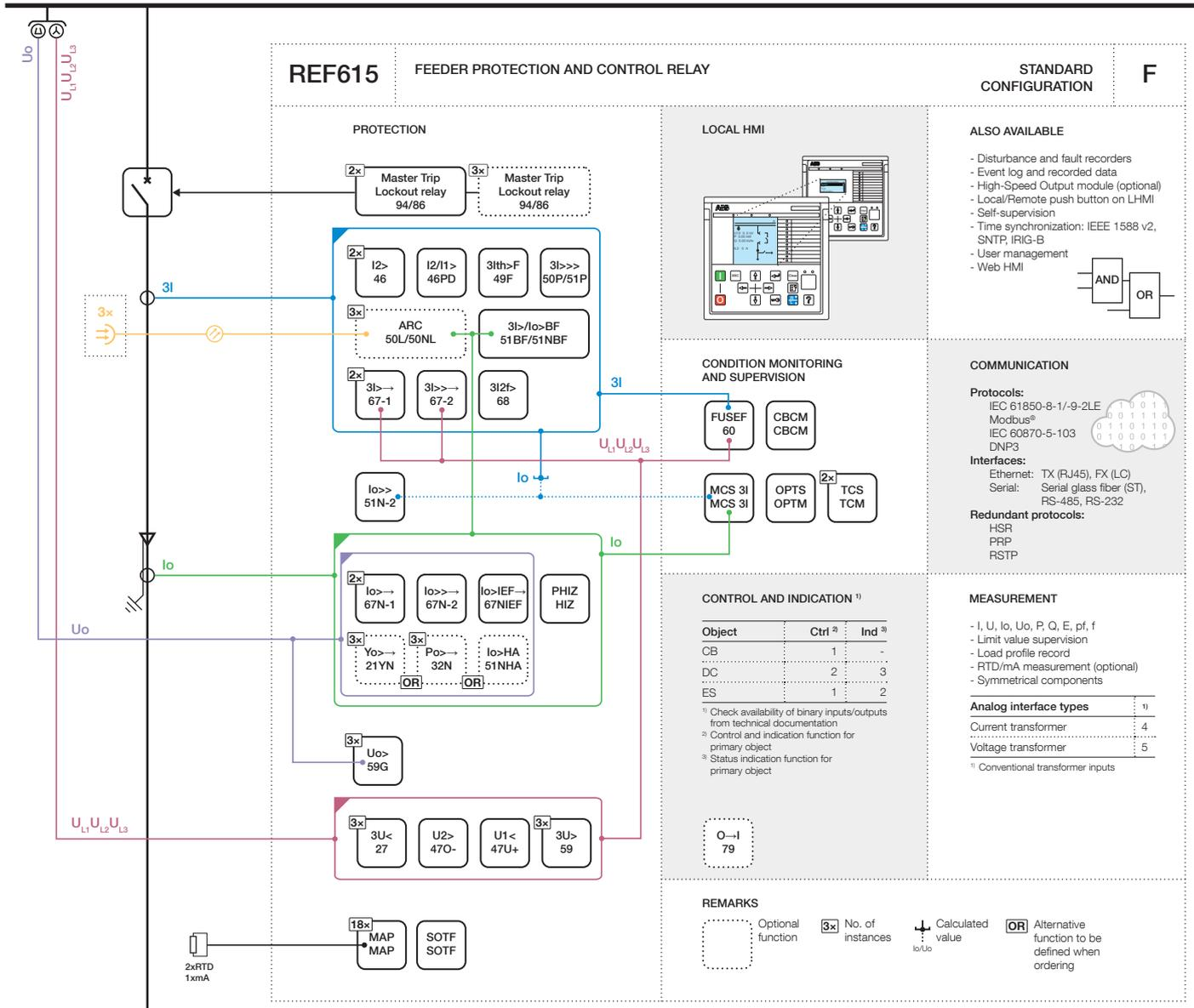
Figure 6. Functionality overview for standard configuration F
