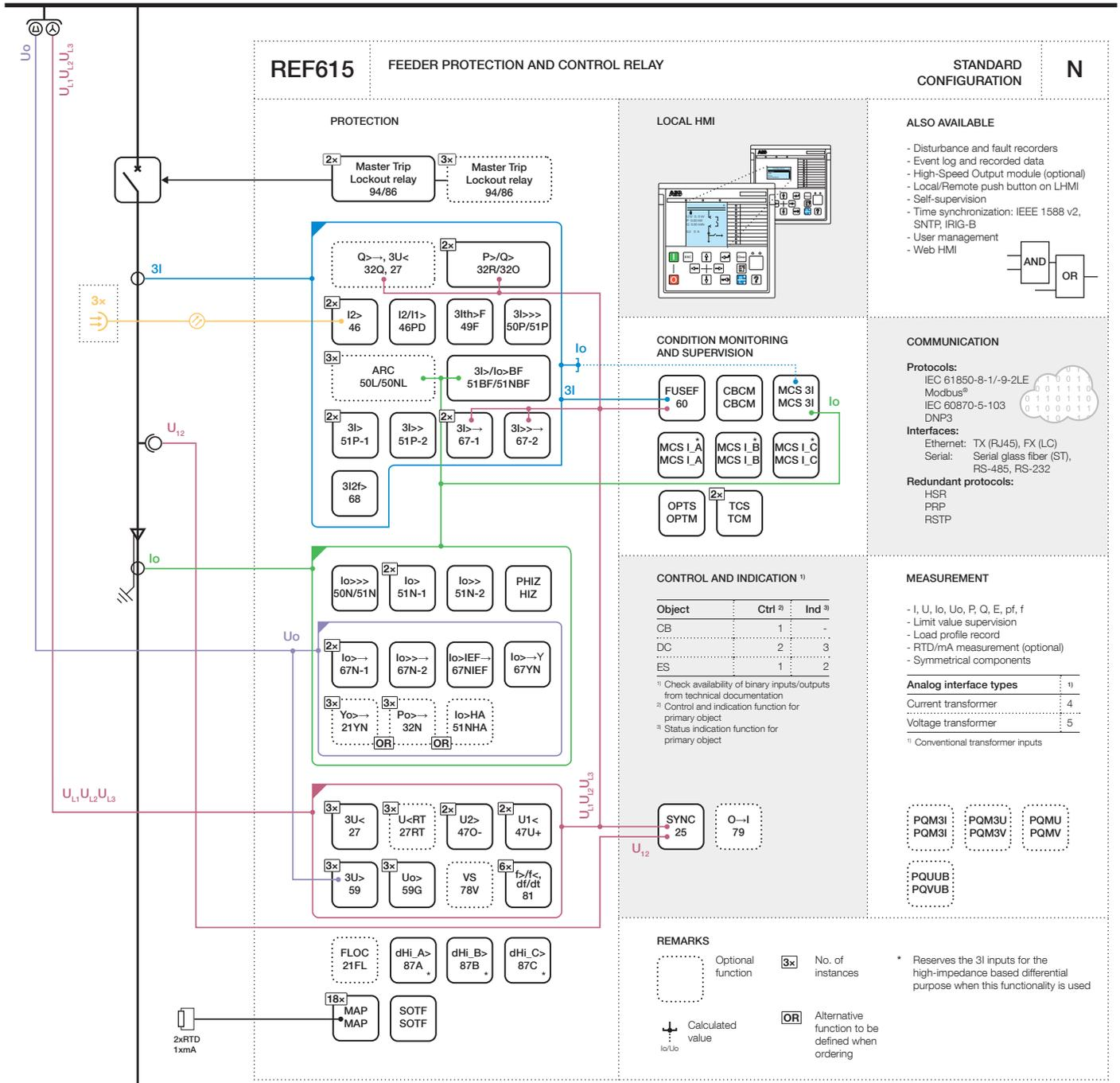
Figure 12. Functionality overview for standard configuration N
