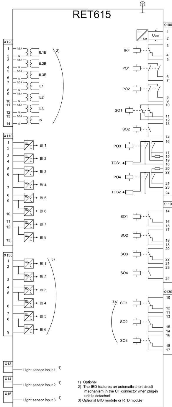
Figure 15. Terminal diagram of standard configuration F
