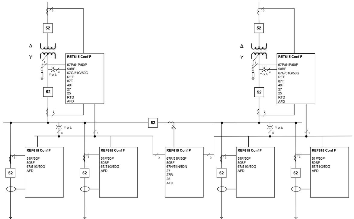
Figure 4 illustrates the protection of the two winding power transformers feeding a double ended substation. In this case configuration F provides the main protection for the transformers: differential protection and low impedance restricted ground fault protection. In addition
