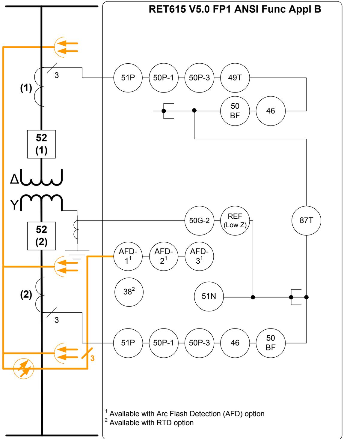
Figure 2. Functionality overview for standard configuration F
