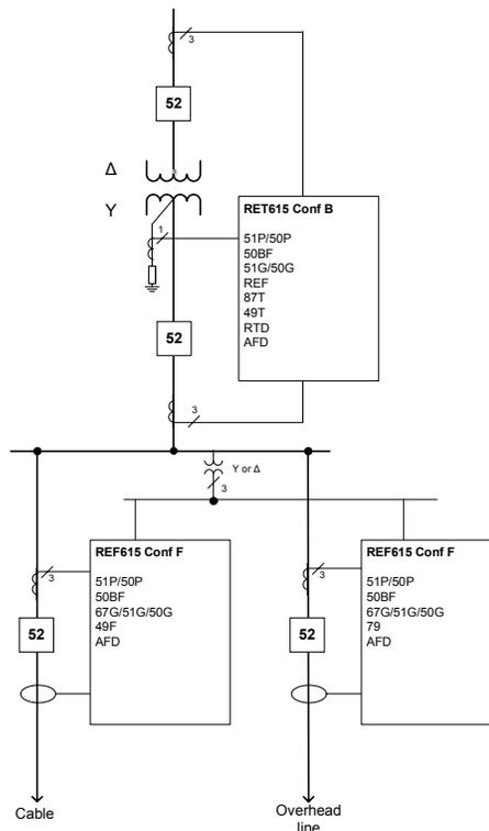
Figure 3. Illustrates the protection of a two winding power transformer with configuration B. The main protection used in this application example is transformer differential protection. Additionally,
