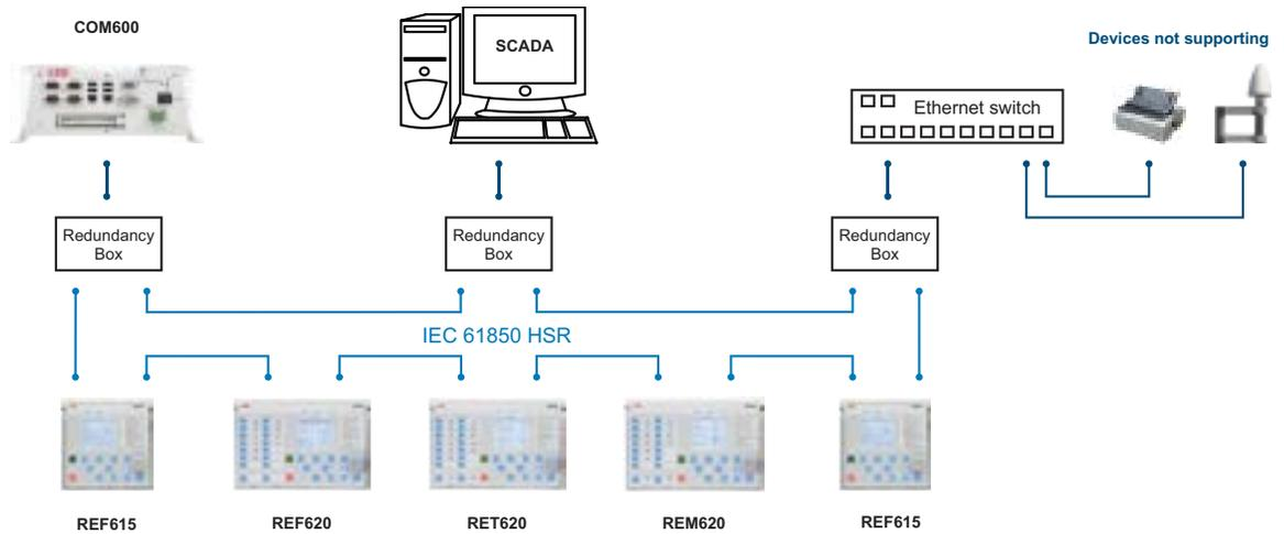
The choice between the HSR and PRP redundancy protocols depends on the required functionality, cost and complexity.
