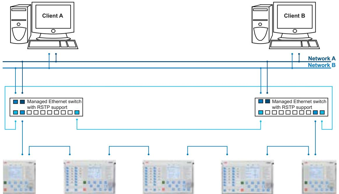
All communication connectors, except for the front port connector, are placed on integrated optional communication modules. The relay can be connected to Ethernet-based communication systems via the RJ-45 connector (100Base-TX) or the fiber optic LC connector (100Base-FX). If connection to serial bus is required, the 9-pin RS-485 screw-terminal can be used. An optional serial interface is available for RS-232 communication.
